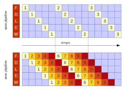
F:fetch; D: Decode; L: load; E:Execute; W:write
