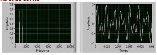
$$V_{dtmf}(t) = v1(t) + v2(t) = 0.7.\sin(2.\Pi.1209.t) + 0.7.\sin(2.\Pi.697.t)$$
